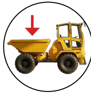
Low the headboard to prevent overloading the skip.
